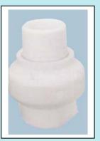
Optimal nozzles for rinsing tanks. Especially suited for CIP systems - no motor source is needed due to the reactionary force the cleaning liquid to rotate the spray head. increase speed of rotation by pressure increase Spray coverage 180<sup>°</sup>, 260<sup>°</sup> and 360<sup>°</sup> 1/2" inside thread material in Plastic Teflon max. operating temp.: 93°C. Flow rate range: 13,5 to 120 l/min.
